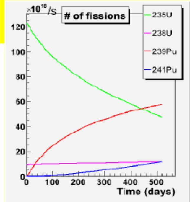
(Modern reactors are built so that they can burn since the beginning admixtures of U and Pu (MOX) since there is “abundance” of Pu, from nuclear weapons which are being dismantled as the consequence of international treaties...)
